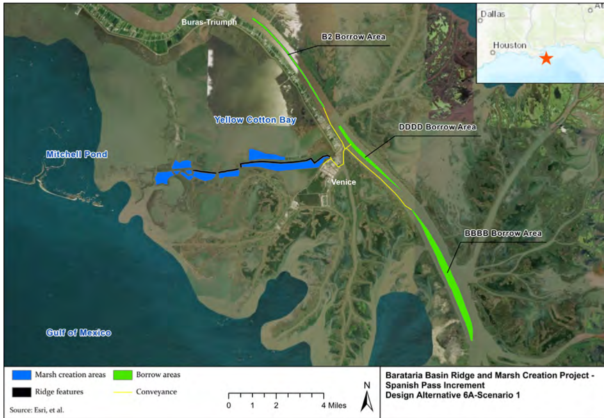
Figure 3-1. Spanish Pass Design Alternative 6A-Scenario 1 with Borrow Areas.
