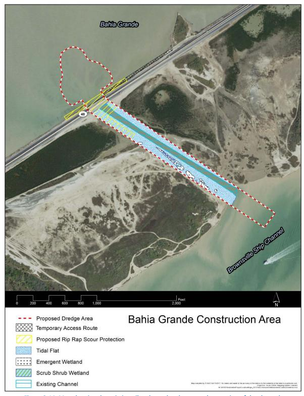
Figure 3-14. Map showing the existing pilot channel and proposed expansion of the channel.
