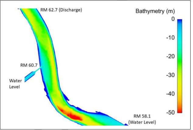
1415 Figure 3.7-2. The lateral bar near the River Mile 60.7 diversion intake (area of shallow bathymetry in front of the 1416 diversion structure) will be monitored routinely with high-resolution velocity and bathymetric surveys along 1417 transects that have been established for design data collection and earlier studies. Figure from (Moffat & Nichol, 1418 2012)
