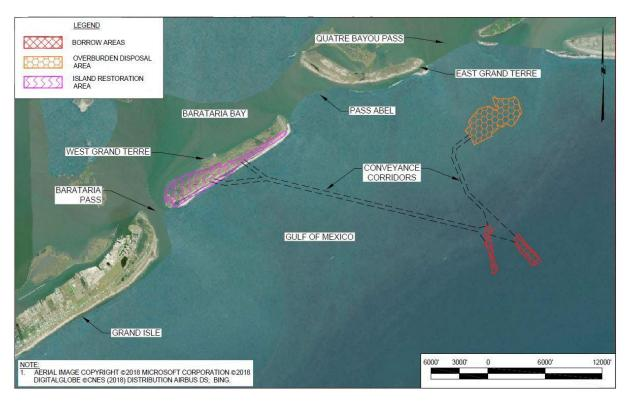
Figure 1. Project location map including the restoration site, borrow area, and pipeline corridor (CEC 2019a).
